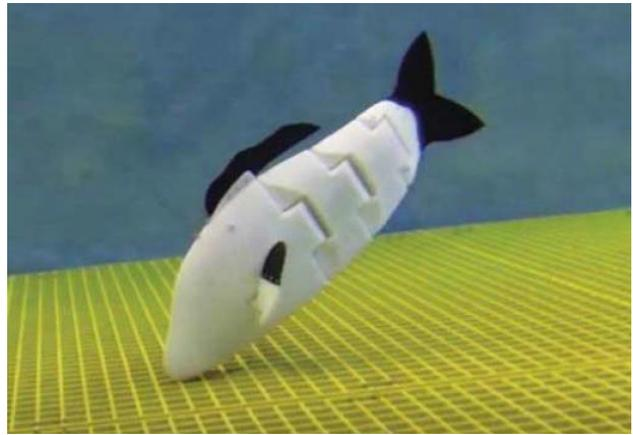
Fig. 4 The CyberFish with tail fin made of three interconnected rigid elements and end-part made of flexible material [12]
